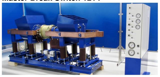
In short circuit laboratories high voltage equipment, for instance a transformer or high voltage switch, is being tested for durability against extreme peak exposures, high voltages and/or high currents.
